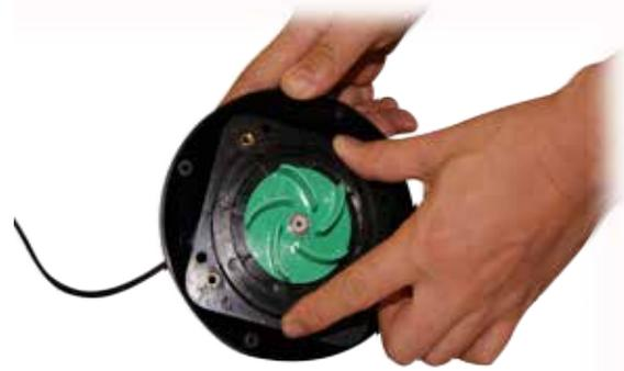
**7** There are pins on the impeller housing that the impeller will click into. The impeller has openings on the back for the pins to click into.
