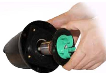
**5** If your impeller and impeller housing have excessive scale build-up, clean with a mild acid, such as white vinegar or non-abrasive calcium, lime and rust remover product using a sponge or soft-bristled brush that won't scratch the stainless steel. Removing scale build-up will allow your pump to run like new again.
