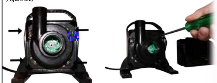
**3** Pull the pump cover off the impeller housing.
