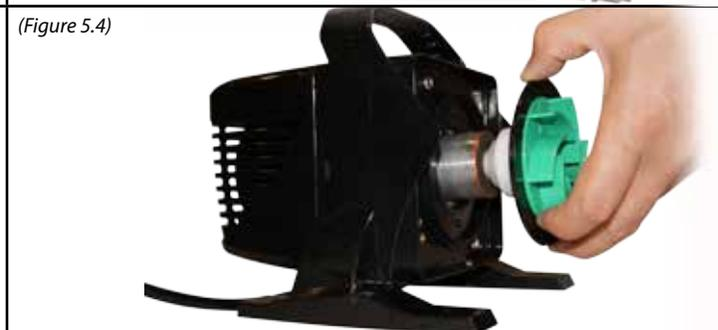
**5** If your impeller and impeller housing have excessive scale build-up, clean with a mild acid, such as white vinegar or non-abrasive calcium, lime and rust remover product using a sponge or soft-bristled brush that won't scratch the stainless steel. Removing scale build-up will allow your pump to run like new again.
