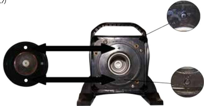
**8** Place the pump body cover to the pump body by aligning the screw holes and screw all 8 screws back in to the pump body.
