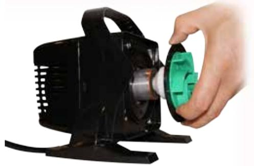
**7** There are pins on the impeller housing that the impeller will click into. The impeller has openings on the back for the pins to click into.
